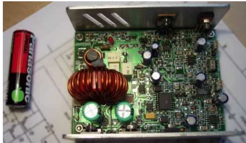
Complete 400W Full-Range Class-D Amplifier Module (Courtesy of ColdAmp)
