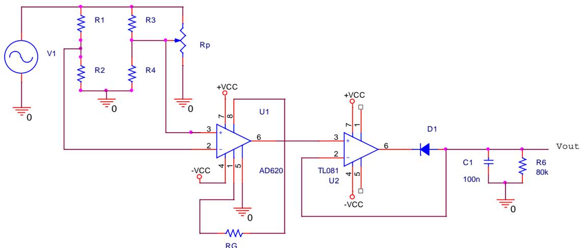
**Figure 1.2** *Wheatstone Bridge, Instrumentation Amplifier and Precision Rectifier*
