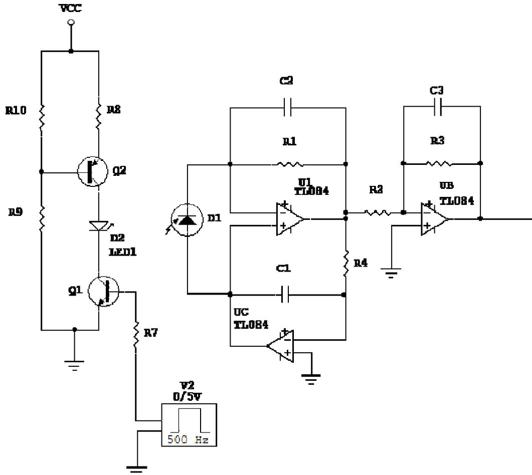
Figure 3.3. Scheme of the proposed conditioning circuit
