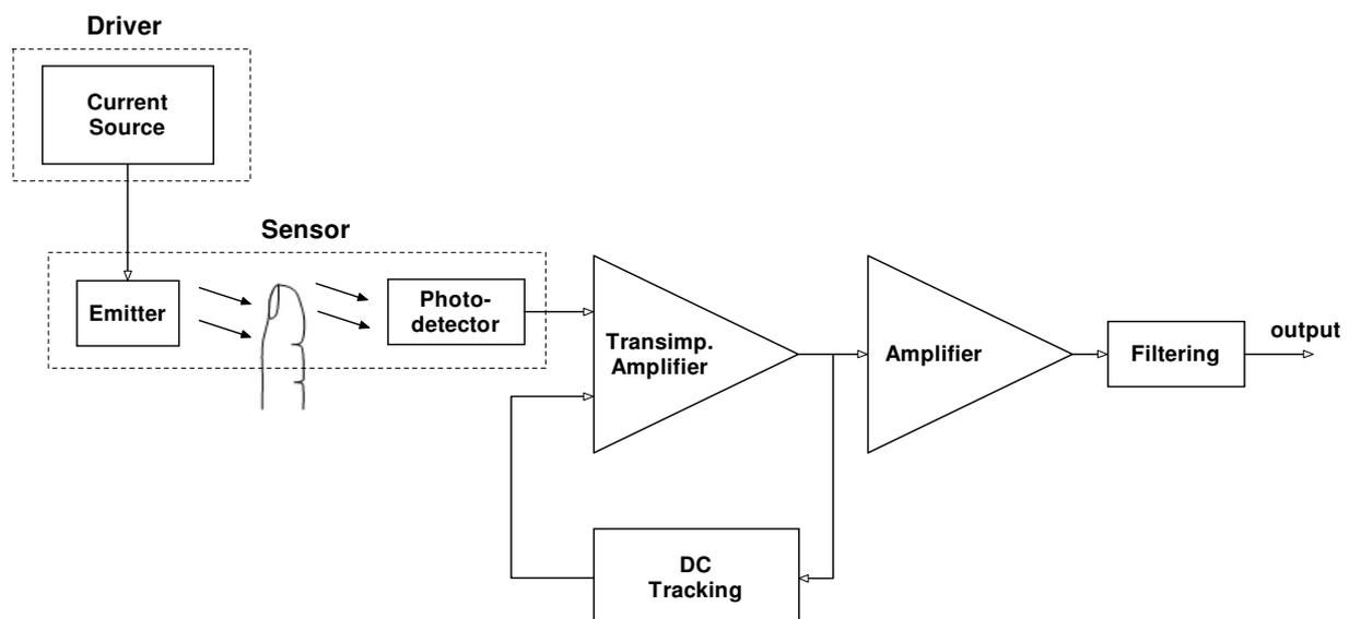
Figure 3.1: Block diagram of the sensor system
