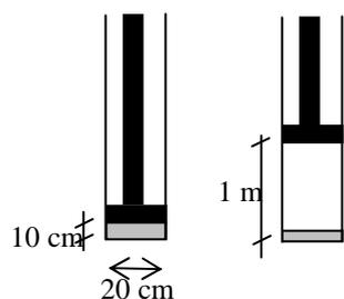
a) As the piston moves a vacuum is created in the cavity the piston leaves below. Water evaporates to fill the vacuum until water vapor pressure equals the equilibrium value at 80 °C. You can look in the web [http://www.engineeringtoolbox.com/water-thermal-properties-d\\_162.html](http://www.engineeringtoolbox.com/water-thermal-properties-d_162.html)
