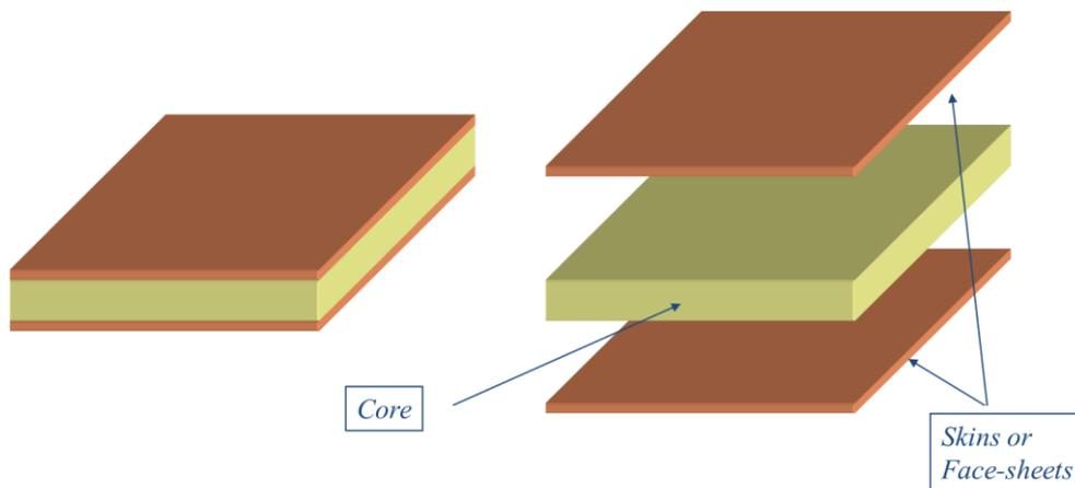
Figure 4. Definition of a sandwich structure
