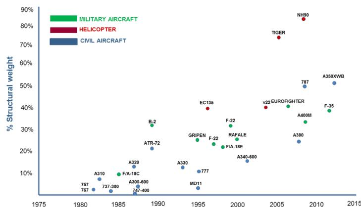
Figure 1. Evolution of the percentage of composite material in the structural weight of aircraft.
