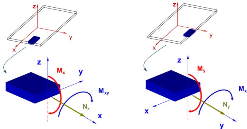
Figure 3. Applied forces per unit length in a laminate
