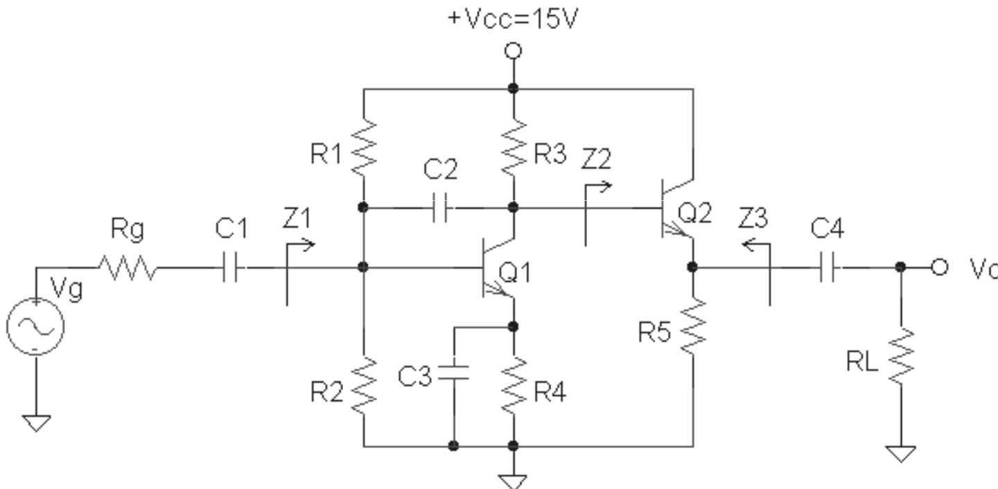
$$R_g = 5 \text{ k}\Omega; R_1 = 30 \text{ k}\Omega; R_2 = 15 \text{ k}\Omega; R_3 = 10 \text{ k}\Omega; R_4 = 8,8 \text{ k}\Omega; R_5 = R_L = 4,7 \text{ k}\Omega$$
