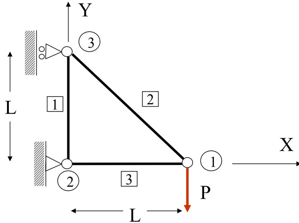
$$\begin{Bmatrix} 0 \\ -P \\ 0 \end{Bmatrix} = \begin{bmatrix} \frac{k}{\sqrt{2}} + k & -\frac{k}{\sqrt{2}} & \frac{k}{\sqrt{2}} \\ -\frac{k}{\sqrt{2}} & \frac{k}{\sqrt{2}} & -\frac{k}{\sqrt{2}} \\ \frac{k}{\sqrt{2}} & -\frac{k}{\sqrt{2}} & \frac{k}{\sqrt{2}} + k \end{bmatrix} \begin{Bmatrix} u_{X1} \\ u_{Y1} \\ u_{Y3} \end{Bmatrix}$$
