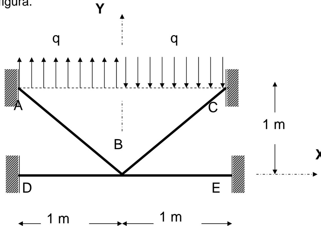
DATOS:  $EI = 10^2 \text{ kN.m}^2$ ,  $EA = 10^5 \text{ kN}$
