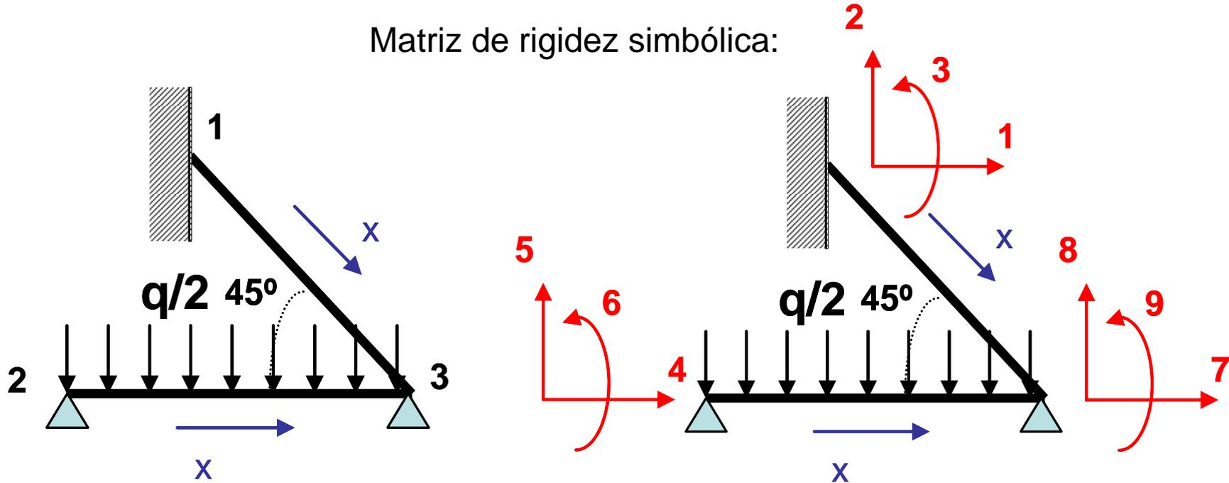
$$[K] = \begin{bmatrix} K_{11}^{barra\ 1-3} & \Omega & K_{12}^{barra\ 1-3} \\ \Omega & K_{11}^{barra\ 2-3} & K_{12}^{barra\ 2-3} \\ K_{21}^{barra\ 1-3} & K_{21}^{barra\ 2-3} & K_{22}^{barra\ 1-3} + K_{22}^{barra\ 2-3} \end{bmatrix}$$
