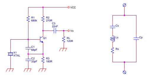
DATA: VCC=5V; Q1:  $I_{CQ}$ =0,75mA,  $V_{BE}$ =0,7V,  $h_{FE}$ =125,  $V_{T}$ =25mV; XTAL: Cs=0,007pF, Ls=100,55mH, Rs=40 $\Omega$ , Cp=5pF, fs=5,999MHz, fp=6,003MHz;
