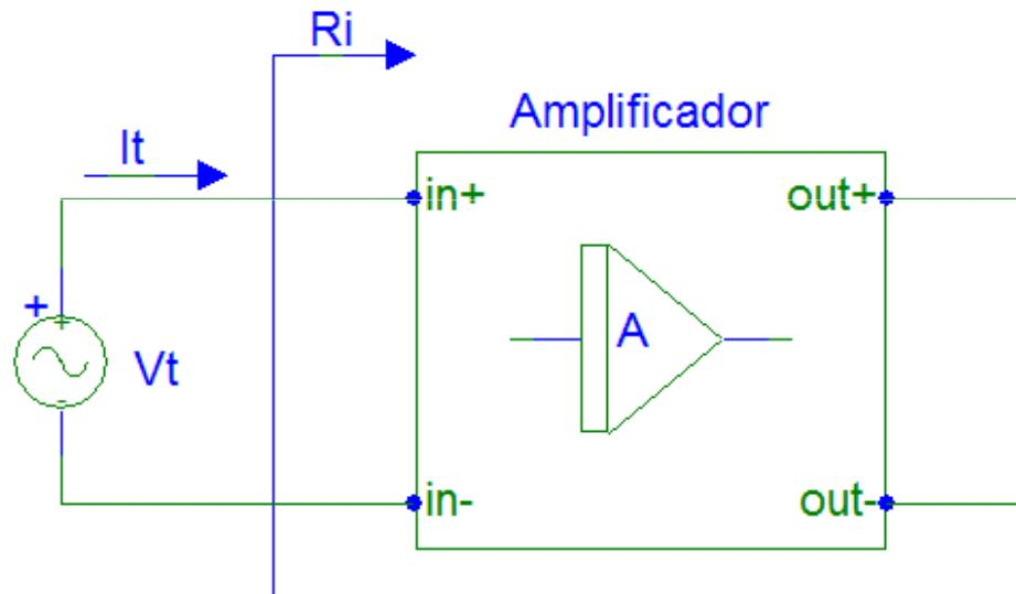
$$R_i = \left. \frac{V_t}{i_t} \right|_{R_L \rightarrow \infty}$$
