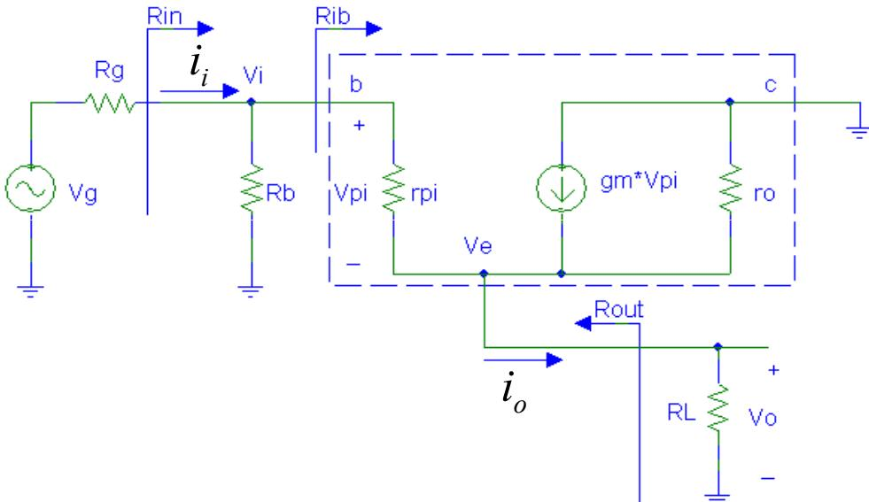
$$G_v = \frac{V_o}{V_g} = \frac{(1+\beta_o) \cdot R_{EM}}{r_\pi + (1+\beta_o) \cdot R_{EM}} \cdot \frac{R_{in}}{R_g + R_{in}} \approx 1$$
