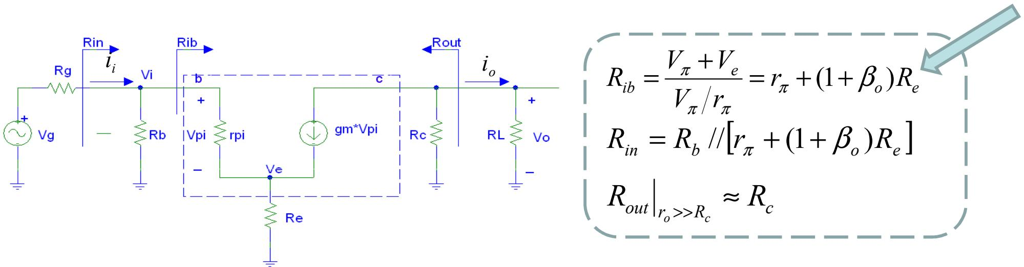
$$R_{ib} = \frac{V_\pi + V_e}{V_\pi / r_\pi} = r_\pi + (1 + \beta_o) R_e$$
