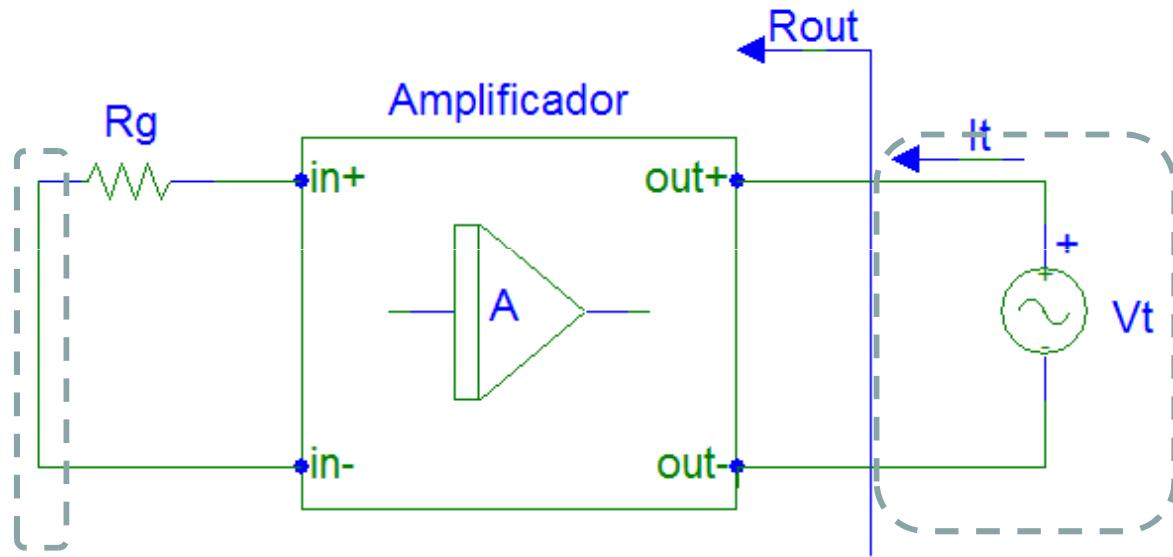
$$R_{out} = \left. \frac{V_t}{i_t} \right|_{V_g=0}$$
