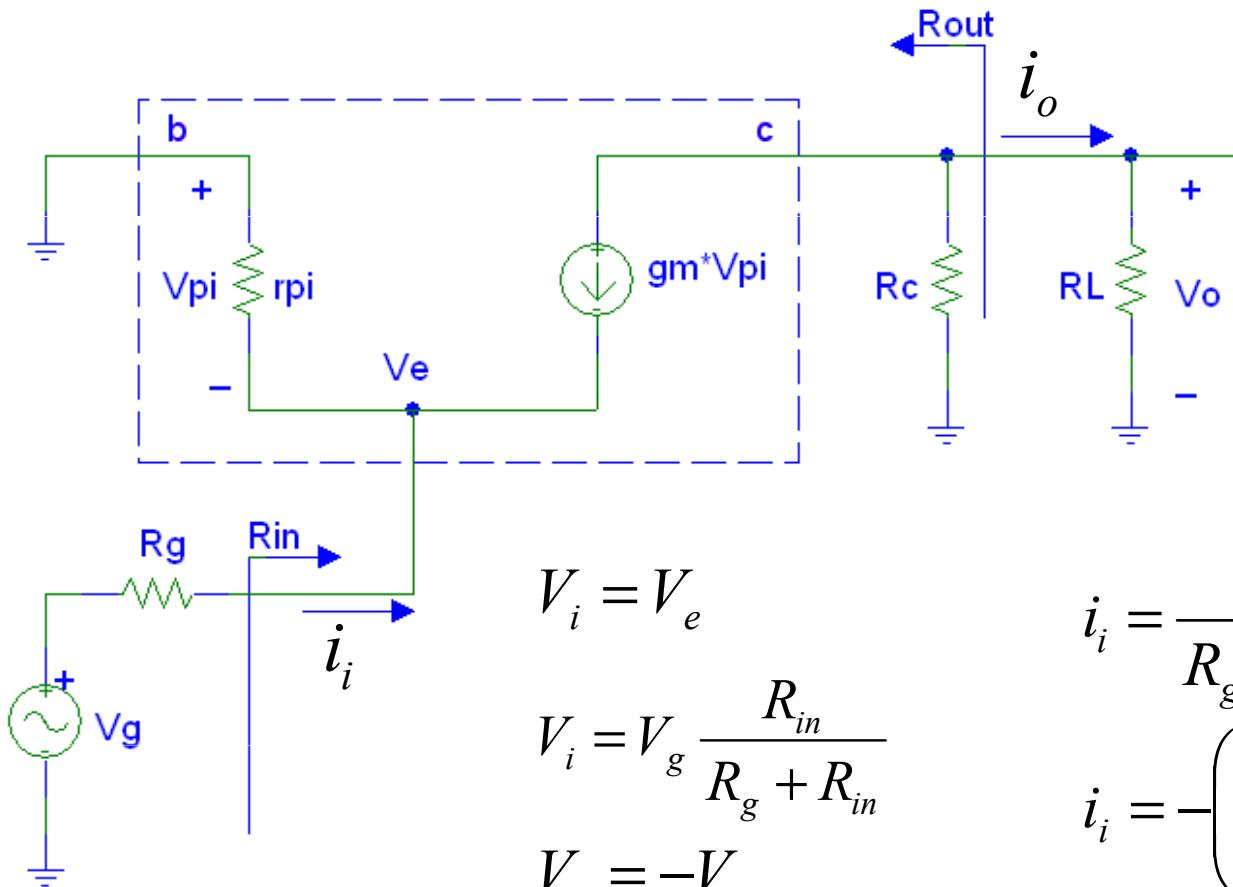
$$V_i = V_g \frac{R_{in}}{R_g + R_{in}}$$
