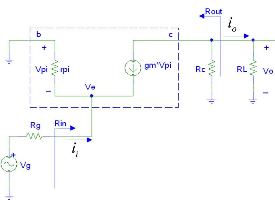
$$G_v = \frac{V_o}{V_g} = +g_m(R_c // R_L) \frac{R_{in}}{R_g + R_{in}}$$
