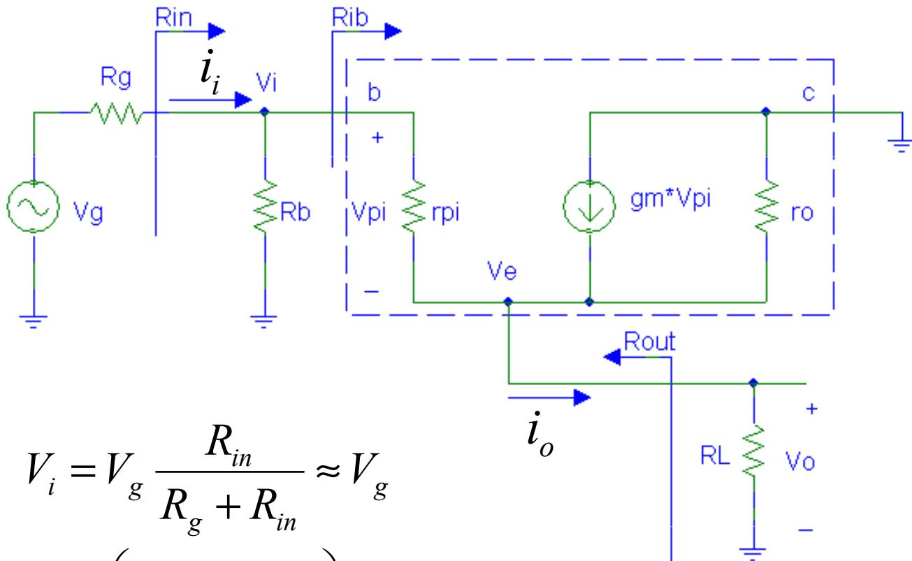
$$V_i = V_g \frac{R_{in}}{R_g + R_{in}} \approx V_g$$
