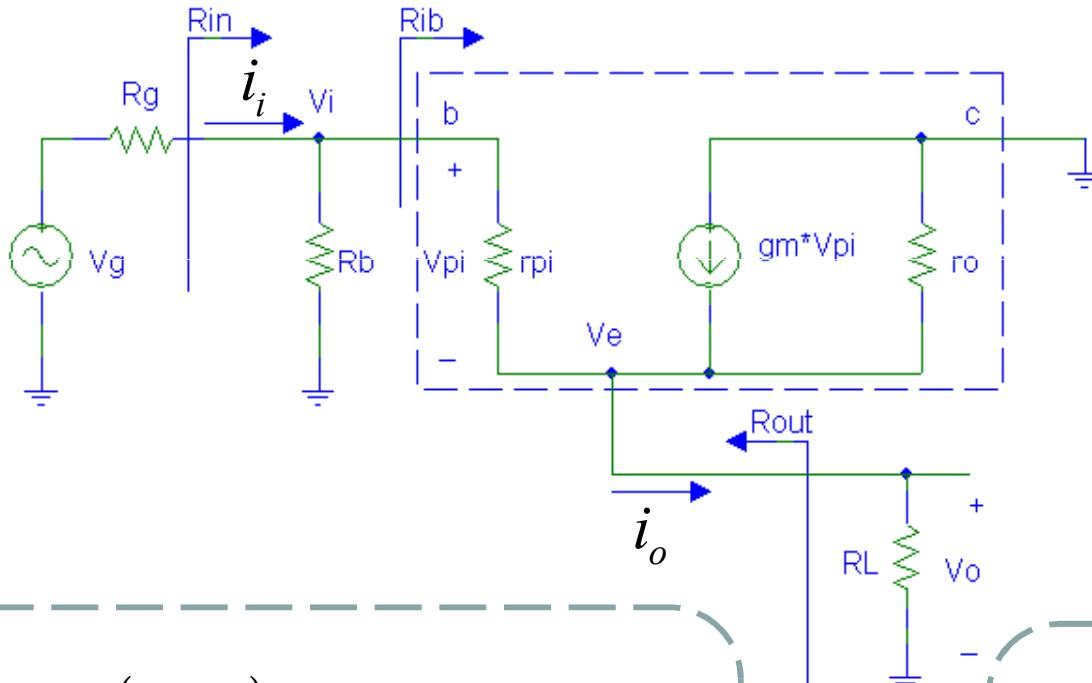
$$A_v = \frac{V_o}{V_i} = \frac{(1 + \beta_o) \cdot R_{EM}}{r_\pi + (1 + \beta_o) \cdot R_{EM}}$$
