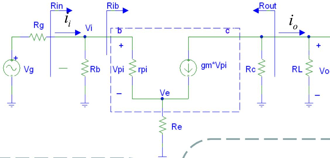
$$A_v = \frac{V_o}{V_i} = -\frac{\beta_o (R_c // R_L)}{r_\pi + (1 + \beta_o) R_e}$$
