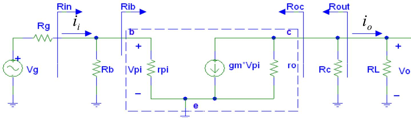
$$A_v = \frac{V_o}{V_\pi} = -g_m (r_o \parallel R_c \parallel R_L)$$
