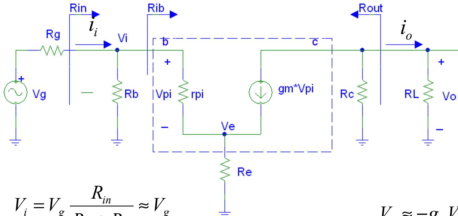
$$V_i = V_g \frac{R_{in}}{R_g + R_{in}} \approx V_g$$
