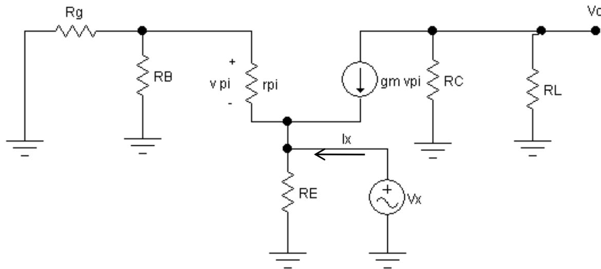
$$R_E^\infty = R_E \parallel \frac{r_\pi + (R_g \parallel R_B)}{1 + \beta_0}$$
