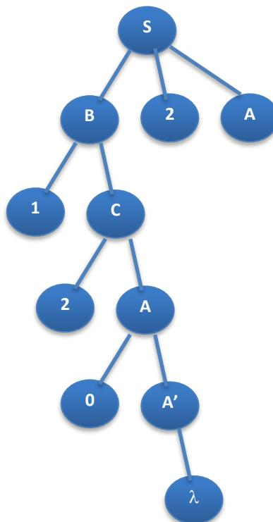
The top of the stack is a terminal symbol (2), but it is not the same that the current token (\$). Thus, an error is generated. The sentence 120 is not recognized.
