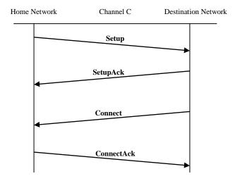
From the home network a **Setup message** is sent to the destination network indicating that it wants to establish a communication with a **SetupAck** message as acknowledgment of the received **Setup** message. Once the destination network terminal accepts the call request, it must send a **Connect message** to the terminal of the source network. The source network must respond with a **ConnectAck** as an acknowledgment of the received Connect message.
