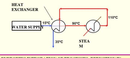
ENERGETIC INTEGRATION OF PROCESSES: REDUCTION IN STEAM AND COOLING WATER
