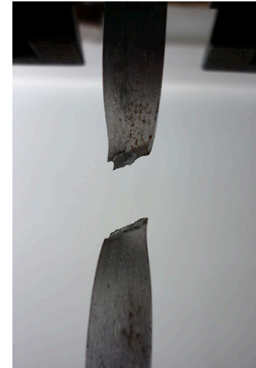
Side view of a flat broken tensile sample, showing the necking and the 45° direction of fracture.
