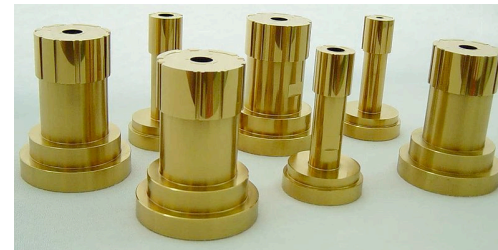
http://commons.wikimedia.org/wiki/File:TiNCoatedPunches_NanoShieldPVD_Thailand.JPG punching dies and cutting tools
