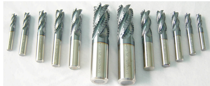
Aluminium Titanium Nitride coated Endmill recoated tools http://commons.wikimedia.org/wiki/File:AlTiNCoatedEndmill_NanoShieldPVD_Thailand.JPG
