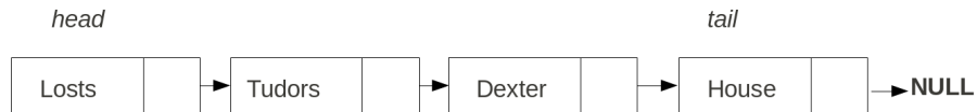
Figure 1: Example of a singly linked list containing my favorite series order by preference. Each node contains a reference to the name of a TV serie and a reference to the next node (the following TV serie). The next reference of the last node (tail) links to null .
