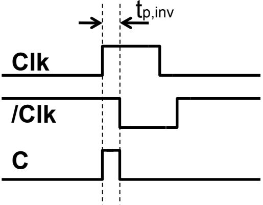
Bad solution due to technology. Inverter delay is not controllable.
