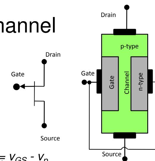
$$i_D = K(V_{GS} - V_p)^2, \quad K = I_{DSS} / V_p^2$$
