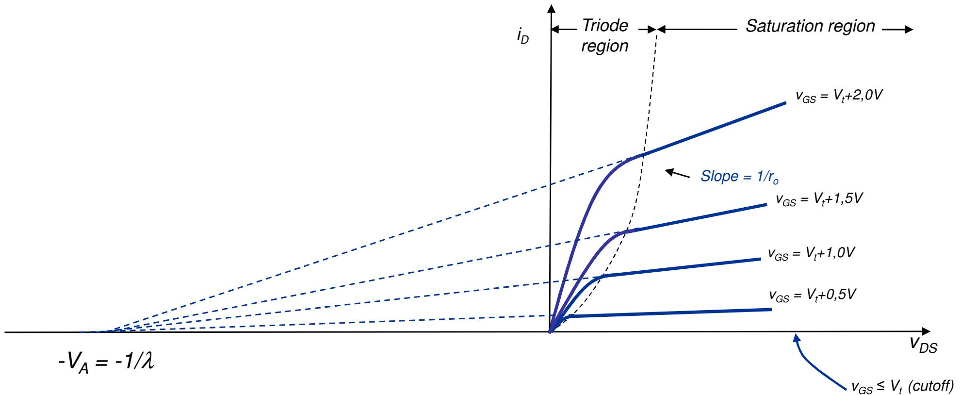
$V_A$  is the channel modulation voltage, producing a similar effect to the Early voltage in BJT devices.
