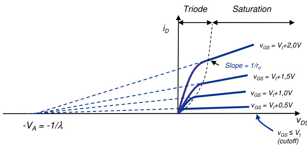
$$\frac{1}{r_o} = \frac{\partial i_D}{\partial v_{DS}} \approx \lambda I_D = \frac{I_D}{V_A}$$
