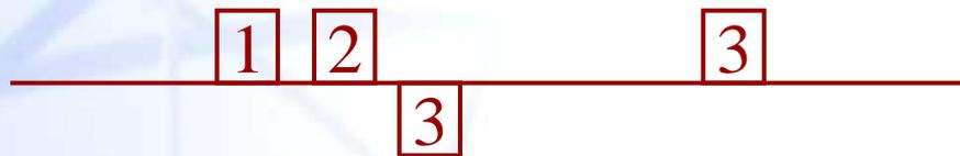
$$U = \frac{T_{tx}}{T_{total}} = \frac{T_{tx}}{N_r * (T_{tx} + 2T_{prop}) + T_{tx}} = \frac{1}{N_r(1 + 2a) + 1}$$
