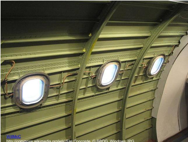
The direct load paths are interrupted and as a result the structure around the cut-out must be reinforced to maintain the required strength
