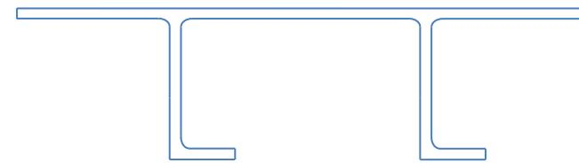
Wing skins are machined from a thick plate to obtain the skin-stringer geometry
