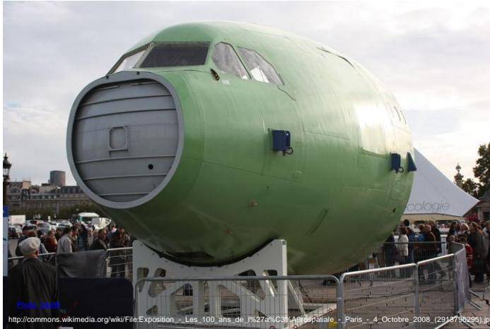
The fuselage function is to carry the payload and support many the aircraft system. They connect the other structural element (wing and empennage)
