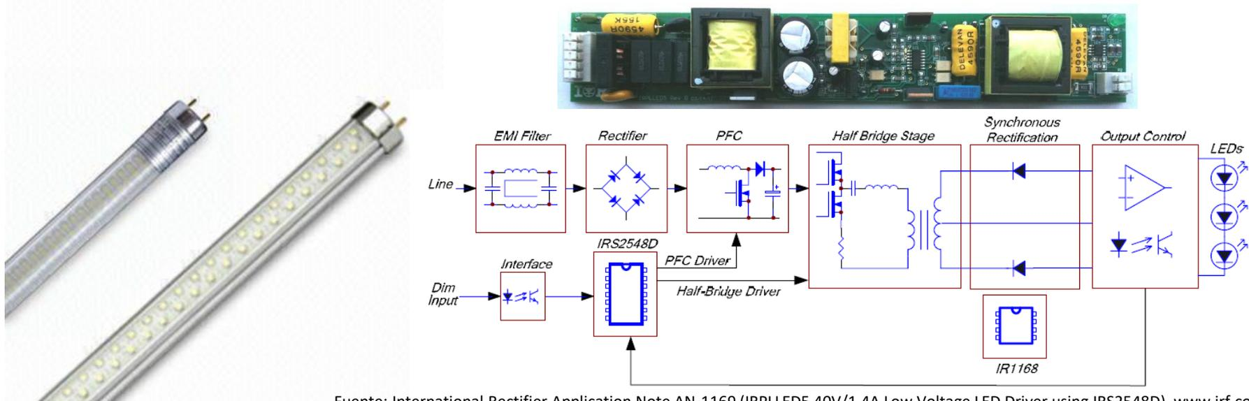
Fuente: International Rectifier Application Note AN-1169 (IRPLED5 40V/1.4A Low Voltage LED Driver using IRS2548D), www.irf.com (Sept'11)
