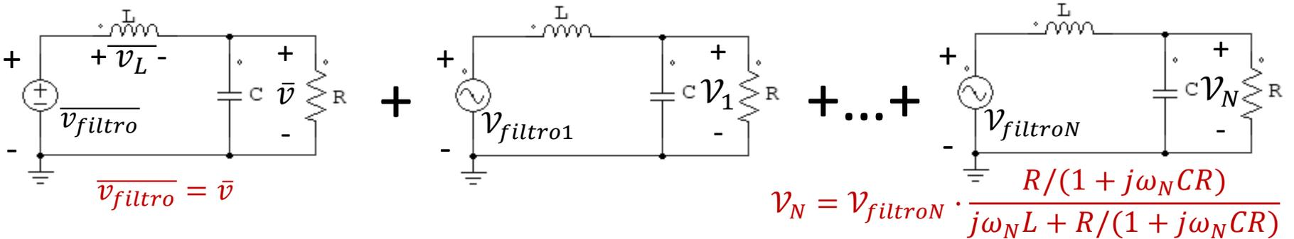
$$V_{ef}^2 = \bar{v}^2 + \left(\frac{|\mathcal{V}_1|}{\sqrt{2}}\right)^2 + \dots + \left(\frac{|\mathcal{V}_N|}{\sqrt{2}}\right)^2$$
