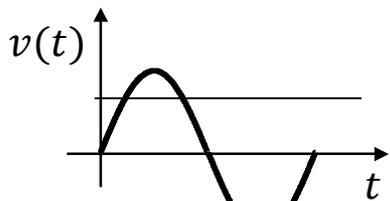
$$V_{ef} = \frac{V_{max}}{\sqrt{2}}$$
