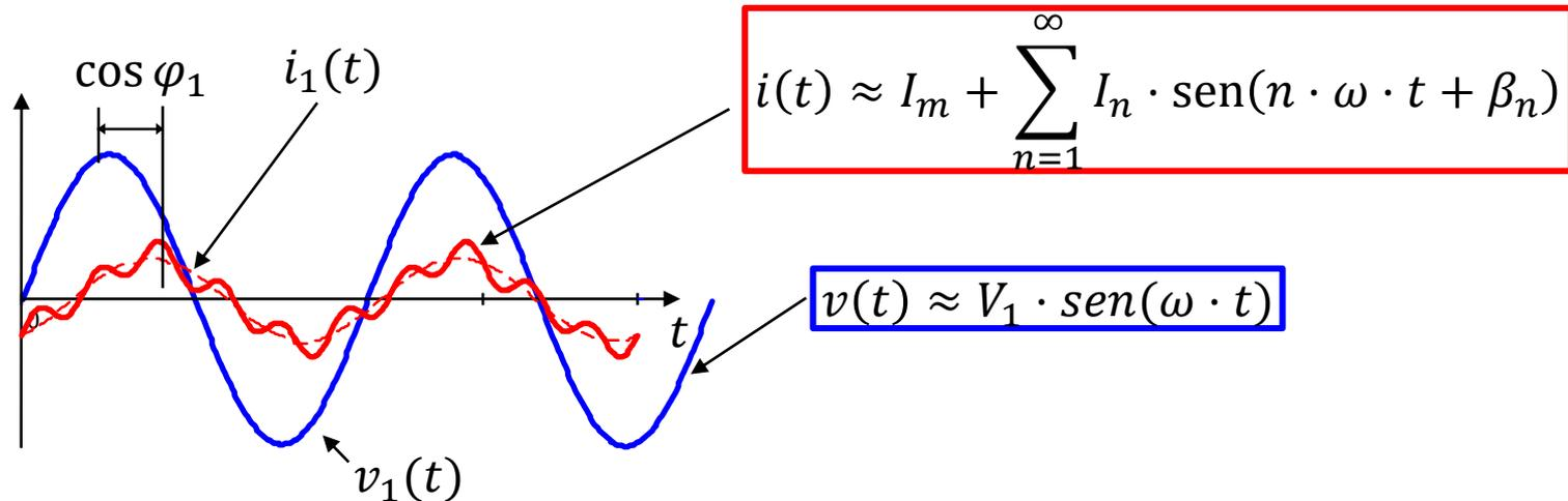
$$FP = \frac{P}{S} = \frac{V_{ef} \cdot I_{1ef} \cdot \cos(\varphi_1)}{V_{ef} \cdot I_{ef}} = \underbrace{\frac{I_{1ef}}{I_{ef}}}_{F_D} \cdot \underbrace{\cos(\varphi_1)}_{F_\varphi} = \frac{1}{\sqrt{1 + DAT^2}} \cdot \cos(\varphi_1)$$
