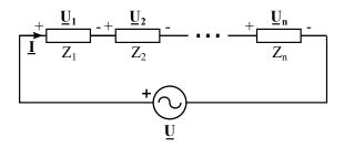
The voltage divider equation is also valid in the frequency domain. The phasor voltage across impedance k is:
