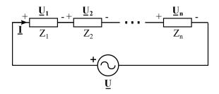
The set of n impedances can be redrawn as an equivalent impedance  $Z_{eq}$
