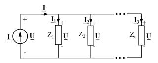
The set of n impedances can be redrawn as an equivalent impedance  $Z_{eq}$
