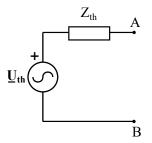
The methods that can be followed to obtain the parameters of the equivalent are analogous to the ones studied for DC circuits.
