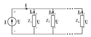
The current divider equation is also valid in the frequency domain. The phasor curretn through across impedance k is:
