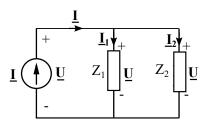
The power supplied by the source equals the sum of the complex power absorbed by the impedances  $Z_1$  and  $Z_2$ .
