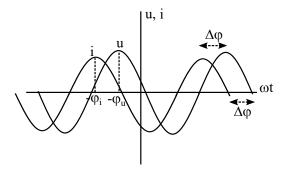
$\Delta \varphi_{u,i} < 0$ : voltage lags current and current leads voltage.
