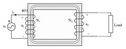
Transformers are based in two coupled inductors with different number of turns. The **transformation relation** is:
