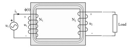
If the number of coils of the two inductors is different, the voltage  $u_2$  differs from  $u_1$ . Transformation relation:
