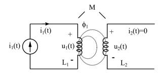
**Mutual inductance coefficient** (M): Degree of coupling between the inductors. It is measured in [H] in the SI.
