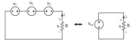
The output voltage of the equivalent voltage source is the sum of the voltages of the individual sources taking into account their polarity
