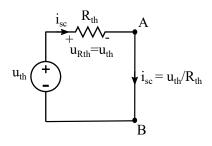
As both circuits are equivalent  $i_{sc}$  is the current flowing through a short-circuit placed between A and B
