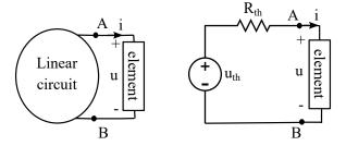
The current flow and the voltage drop across the element is identical in both cases
