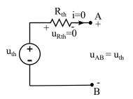
The analysis of the original circuit without connecting anything between A and B provides the value of  $u_{th}$
