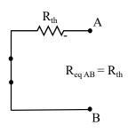
The equivalent resistance between terminals A and B is  $R_{th}$
