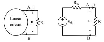
If we redraw the circuit as its Thevenin equivalent we can calculate the R that absorbs the maximum power from the circuit as:
