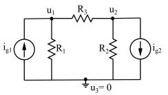
2. Set a "reference node" in which u=0 and then apply KCL to the remaining nodes of the circuit, considering that the voltage level of each node is the correspondent nodal voltage.
