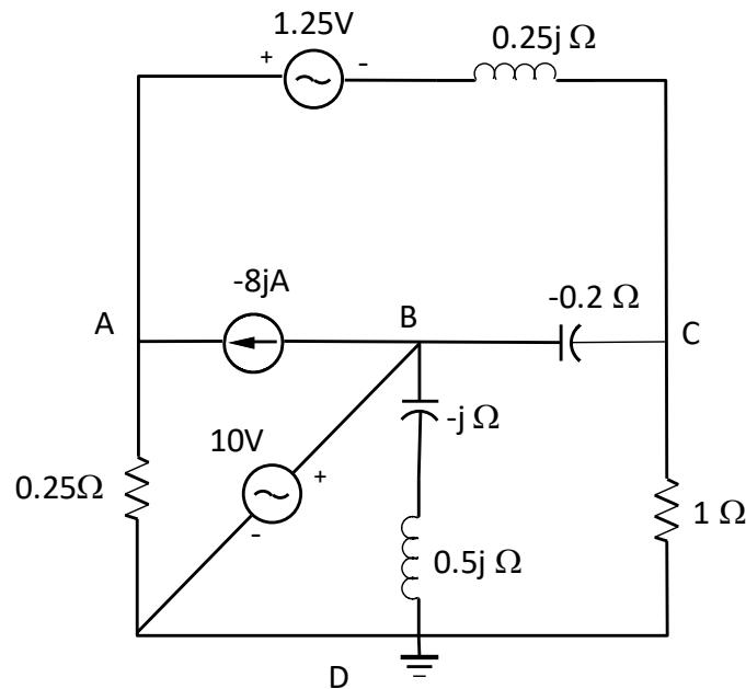
We can transform the real voltage source into a real current source to facilitate the analysis of the system with nodal method
