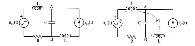
a) Find the Thevenin equivalent in the circuit of the figure on the left between A and B **including all the elements of the circuit in it**. Draw the equivalent indicating the obtained values for the parameters. (6 points)
