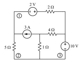
a) Write the equations for the **mesh current method** for the circuit in the figure. (Label the mesh currents with the names provided in the figure and take the mesh currents in clockwise direction). (2.5 points)
