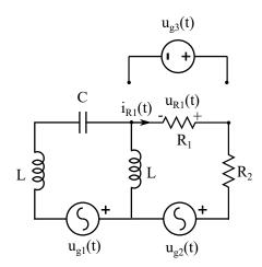
a) Solve the circuit using mesh analysis and calculate the branch currents of the circuit. Write the equations in matrix form and the phasors mesh currents below. (4 points)
