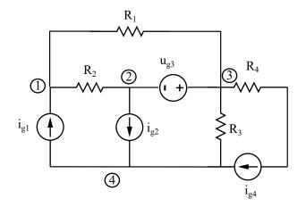
a) Apply nodal analysis to solve the circuit taking 4 as reference node. Write the nodal equations and solve them to find the node voltages (5 points)
