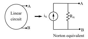
For the calculation of the Norton equivalent of a circuit the sources transformation rules can be applied.
