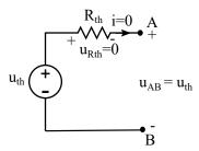
Then, the analysis of the original circuit without connecting anything between A and B provides the value of  $u_{th}$
