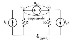
The system must be completed with an additional equation that relates the node voltages with the voltage of the ideal voltage source.
