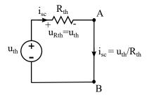
It can be seen that the voltage drop across the resistor  $R_{th}$  equals  $u_{th}$  (we just have to apply KVL to the circuit). Then, applying Ohm's law:
