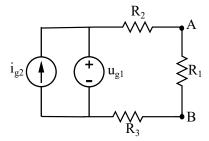
Remember that calculating the Thevenin equivalent of the circuit means determining what couple of values  $u_{th}$  and  $R_{th}$  make the behaviour of the simplified circuit represented below identical to the one of the initial circuit, from the point of view of the couple of terminals A B.
