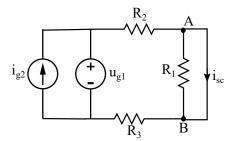
Our goal is to calculate the current  $i_{sc}$  flowing from A to B. We could use any method of analysis to this end.
