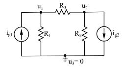
2. We apply KCL to each node of the circuit considering that the voltage of each node is the correspondent node voltage:
