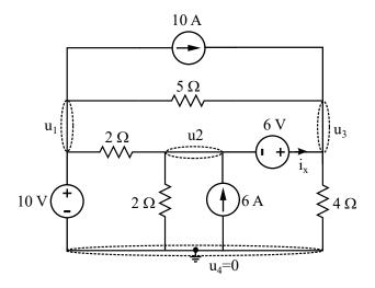
We apply KCL to nodes 1, 2 and 3 and write the nodal equations:
