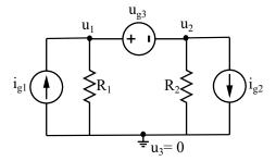
In this case we can not redraw the voltage source as a current source and can not identify the voltage of the source with any of the nodal voltages either.
