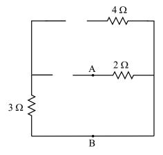
As the resistors of 3 and 4  $\Omega$  are in series with open circuits, the only resistor that contributes to the equivalent resistance is the 2  $\Omega$  one. Thus:
