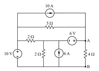
In this example we are requested to calculate the Thevenin equivalent of the whole circuit (ti.e including all the elements of the circuit in it).
