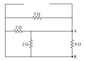
Seen from terminals A B, the four resistors are in parallel. In consequence we calculate Thevenin resistance as:
