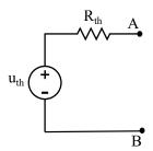
The original circuit and the Thevenin equivalent are equivalent if any element connected between A and B behaves in the same way if we consider the original circuit or the equivalent circuit.
