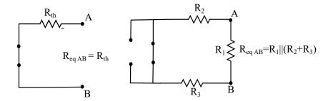
The equivalent resistance between terminals A and B is  $R_{th}$
