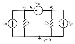
This new unknown will be included in the equations. As we have three unknowns now we need an additional equation to find the node voltages. The additional equation relates the voltage of the ideal voltage source with the node voltages.
