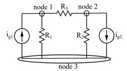
The node voltage method consists of finding the voltage of each node with respect to a "reference node", whose voltage level is zero.
