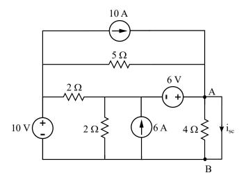
We apply nodal analysis to solve the circuit. Since the  $4\Omega$  resistor is in parallel with a short-circuit and no current will flow through it and it can be eliminated from the circuit. Taking B as reference node, and considering that now  $u_A = u_B$ , it is easy to obtain the remaining node voltage and branch currents.
