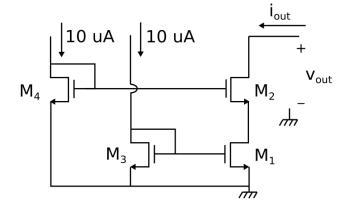
Data:  $\mu_n C_{ox} = 110 \ \mu A/V^2$ ,  $(W/L)_1 = (W/L)_2 = (W/L)_3 = 4$ ,  $(W/L)_1 = 1$ ,  $\lambda = 0.04 \ V^{-1}$
