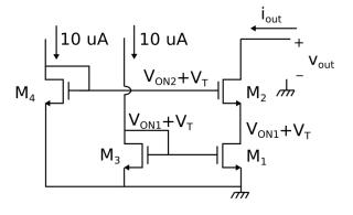
Where V<sub>ON</sub> is the overdrive voltage  $\rightarrow V_{ON} = \sqrt{\frac{2I_D}{\mu n Cox(W/L)}}$
