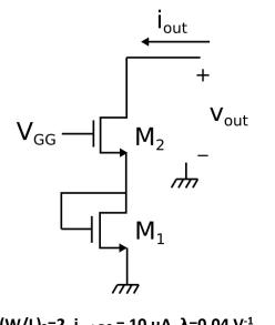
Data:  $\mu_n C_{ox} = 110 \ \mu A/V^2$ , (W/L)<sub>2</sub>=2,  $i_{out,DC} = 10 \ \mu A$ ,  $\lambda = 0.04 \ V^{-1}$
