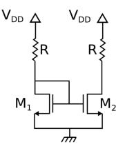
Data:  $V_{DD}$  = 5V, R =100 k $\Omega$ ,  $\mu_n C_{ox}$  = 120  $\mu$ A/V<sup>2</sup>, (W/L)<sub>1</sub>=(W/L)<sub>2</sub>=5, V<sub>th</sub> = 0.8V.
