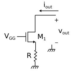
Data: R =50 kΩ,  $\mu_n C_{ox}$  = 110  $\mu$ A/V<sup>2</sup>, (W/L)<sub>1</sub>=2,  $i_{out,DC}$  = 10  $\mu$ A,  $\lambda$ =0.04 V<sup>-1</sup>
