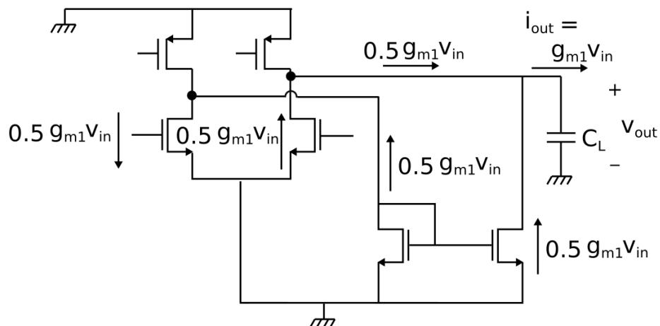
$$R_{out} \approx \frac{1}{1/r_{o4} + 1/r_{o2} + 1/r_{o7}}$$
