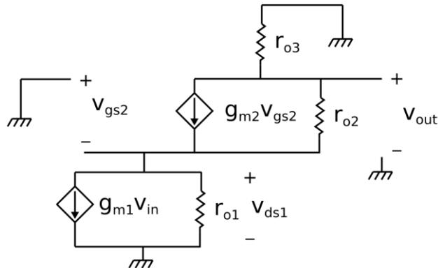
$$A_V = \frac{v_{out}}{v_{in}} \approx -g_{m1}r_{o3} \rightarrow \text{Estimation of } (\frac{W}{L})_1$$
