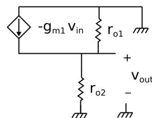
$$A_V = \frac{v_{out}}{v_{in}} \approx -\frac{g_{m1}}{1/r_{o1} + 1/r_{o2}} = -17.56 \text{ V/V}$$
