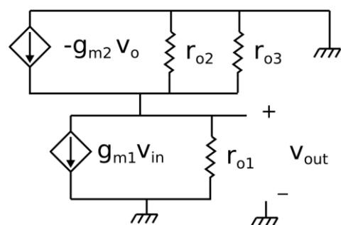
$$A_V = \frac{v_{out}}{v_{in}} \approx -\frac{g_{m1}}{g_{m2}}$$
