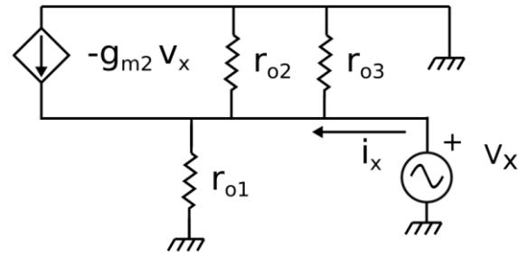
$$R_{out} = \frac{V_x}{i_x} \approx \frac{1}{g_{m2}} = 31.6 \text{ k}\Omega$$
