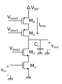
Data:  $\mu_p C_{ox} = 20 \text{ uA/V}^2$ ,  $\mu_n C_{ox} = 60 \text{ uA/V}^2$ ,  $V_{thp} = -0.7 \text{ V}$ ,  $V_{thn} = 0.7 \text{ V}$ ,  $C_L = 3 \text{ pF}$ .
