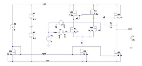
Data: Cc=3pF,I=30 $\mu$ A,(W/L)1=(W/L)2=3,(W/L)3=(w/L)4=5,(W/L)8=(W/L)5=3, (W/L)6=80, (W/L)=18, L<sub>min</sub>=1 $\mu$ m, K<sub>P</sub>=40 $\mu$ A/V,  $\lambda_P$ (L=2 $\mu$ m)=0.02V<sup>-1</sup>, V<sub>tp</sub>=-0.9V,K<sub>N</sub>=120  $\mu$ A/V,  $\lambda_n$  (L=2 $\mu$ m) = 0.02V<sup>-1</sup>, V<sub>tn</sub> = 0.8 V
