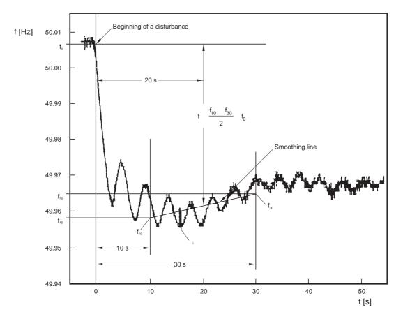
It is assumed that the main part of the PRIMARY CONTROL RESERVE is activated after 20 seconds, while the contribution of SECONDARY CONTROL to the correction of the disturbance will not yet be perceptible.
