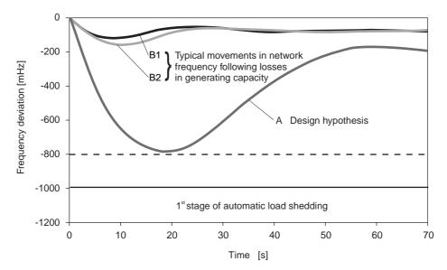
A Loss in generating capacity: P = 3000 MW,  $P_{network} = 150$  GW, self-regulating effect of load: 1% / Hz B1 Loss in generating capacity: P = 1300 MW,  $P_{network} = 200$  GW, self-regulating effect of load: 2 % / Hz B2 Loss in generating capacity: P = 1300 MW,  $P_{network} = 200$  GW, self-regulating effect of load: 1% / Hz
