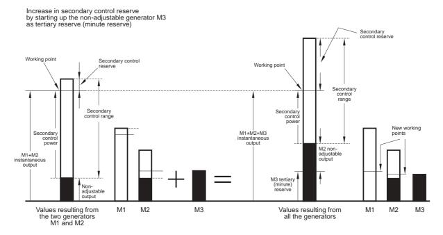
The restoration of an adequate SECONDARY CONTROL RANGE may take, for example, up to 15 minutes, whereas TERTIARY CONTROL for the optimisation of the network and generating system will not necessarily be complete after this time. The timing of the various (partially overlapping) ranges of action of PRIMARY, SECONDARY and TERTIARY CONTROL are shown in the following figure.
