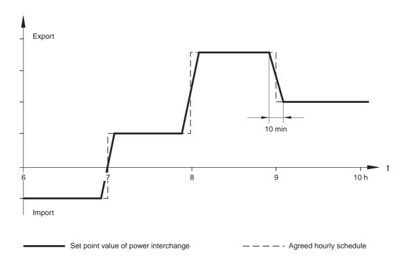
In order to prevent unintentional FREQUENCY DEVIATIONS and major control actions under undisturbed conditions, TRANSMISSION SYSTEM OPERATORS (TSOs) are required to maintain careful compliance with times for programme changes, particularly where changes in the EXCHANGE PROGRAMS of several hundred MW are involved. In particular, care must be taken to ensure that generating capacity is brought on line or disconnected on a staggered basis, particularly for tariff changes at 6 a.m. and 10 p.m.
