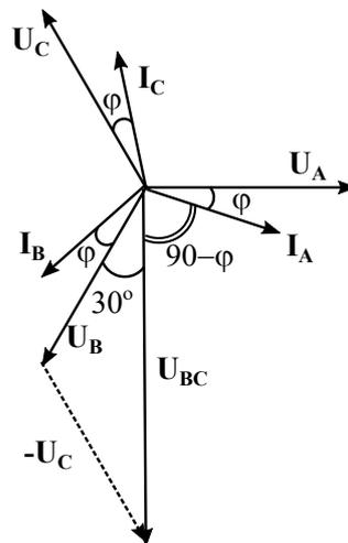
$$W = U_L \cdot I_L \cdot \cos(\widehat{\underline{U}_{BC} \underline{I}_A}) = U_L \cdot I_A \cdot \cos(90 - \varphi) = U_L \cdot I_A \cdot \text{sen}(\varphi) = \frac{Q}{\sqrt{3}} \quad (65)$$
