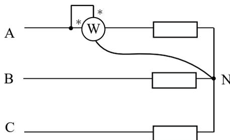
$$W = I_A \cdot U_{AN} \cdot \cos(\widehat{\underline{U}_{AN} \underline{I}_A}) = U_F \cdot I_F \cdot \cos \varphi = \frac{P}{3} \quad (63)$$
