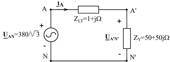
$$\underline{I}_A = \frac{\underline{U}_{AN}}{Z_{LT} + Z_Y} = 1,83 - 1,83j = 2,59 \angle -45^\circ A$$
