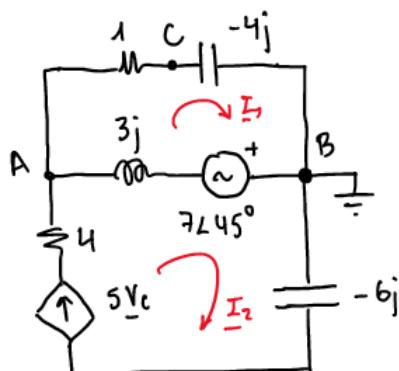
$$v(t) = 7\sqrt{2} \cos(1000t + 45^\circ) \rightarrow V = 7 < 45^\circ \text{ V}$$
