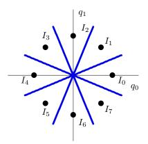
i) For the design of the detector, since the symbols are equiprobable and the noise is Gaussian, the minimum Euclidean distance criterion is applied: the decision region of a symbol are those points in space closer to that symbol than to the rest of the symbols of the constellation, which in this case would be those shown in the previous figure.
