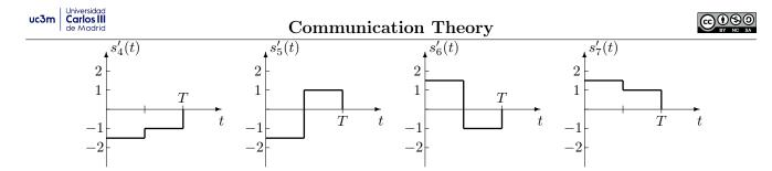
c) The optimal demodulator is based on matched filters or on correlators with the functions that form the orthonormal basis, either of the two options is valid.
