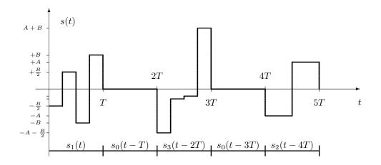
c) To carry out the binary assignment, a Gray code must be used, so that symbols that are at a minimum distance have an assignment that differs by only one bit. This is the assignment that minimizes the bit error rate (BER).
