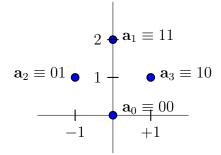
i) Binary assignment has to follow Gray's rule. Given the constellation, a possible binary assignment that meets this rule (it is not the only possible one) would be the one in the figure
