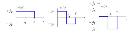
iii) For the demodulator, a bank of two matched filters (in this case causal) or a bank of two correlors can be used, as shown in the figure
