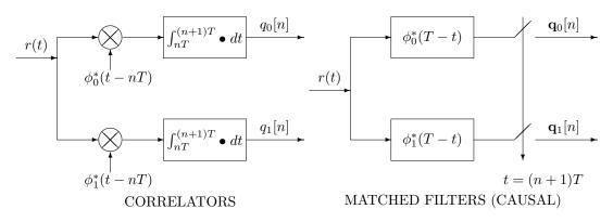
In this case, since the base functions are real, the conjugates are not relevant.
