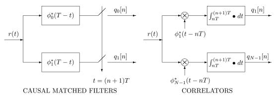
In this case, since the orthonormal basis functions are real, the complex conjugate operators are not relevant.
