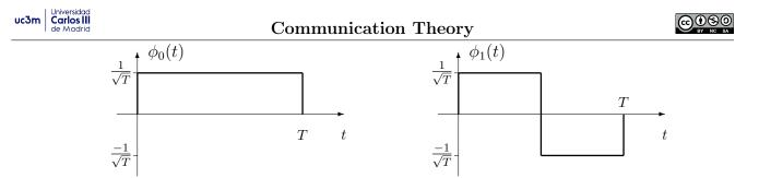
To have them completely defined, the value of T must be determined, and this is related to the transmission rate, since the symbol rate is  $R_s = \frac{1}{T}$  bauds. Symbol rate is related to bit rate through the number of bits per symbol
