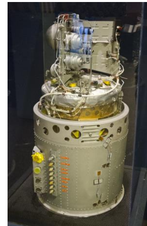
Fuel cell used on the Apollo lunar missions. Museum of the Rockies in Bozeman, Montana
