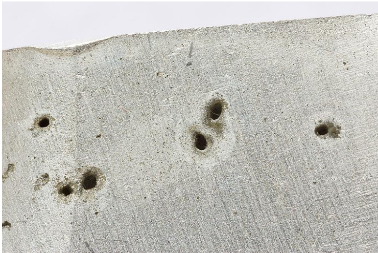
The pitting of aluminium plate
