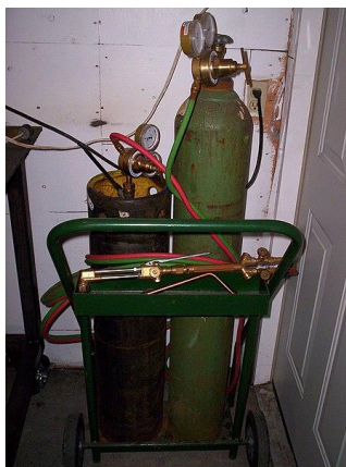
Oxy-Acetylene Gas Welding
