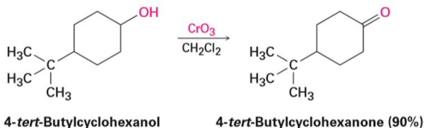
Figure 20. Synthesis of a ketone from a secondary alcohol using \text{CrO}_3 as an oxidant.
