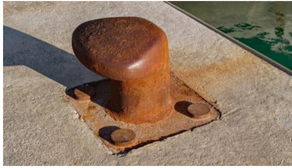
Figure 2. Rusted bollard through uniform attack.
