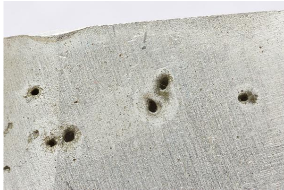
Figure 5. The pitting of aluminium plate.
