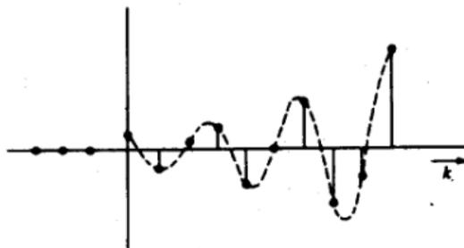
Exponentially expanding sinusoidal sequence
