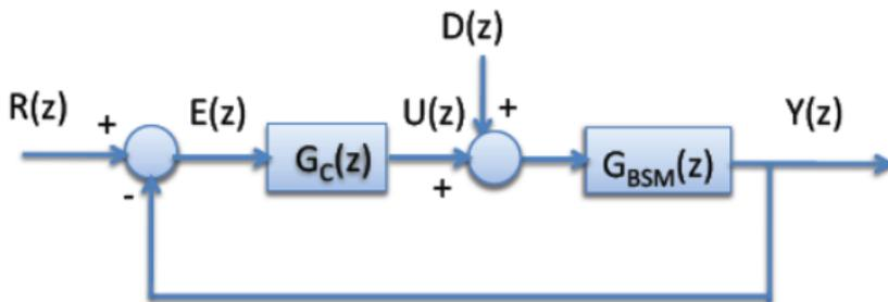
$$\frac{Y(z)}{R(z)} = \frac{G_C(z)G_{BSM}(z)}{1 + G_C(z)G_{BSM}(z)} \quad \frac{Y(z)}{D(z)} = \frac{G_{BSM}(z)}{1 + G_C(z)G_{BSM}(z)}$$
