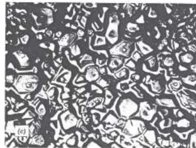
Fig. 10.40. (a) Surface of solid-liquid composite with varying amounts of liquid phase. (b) Drop of liquid between two solid spheres exerts pressure to pull them together. (c) Surface of forsterite ceramic showing liquid capillary depression between crystals.
