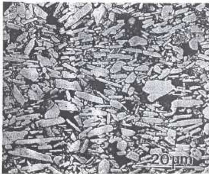
Fig. 5.20 Optical micrograph of an 88% alumina showing alignment of the alumina grains in an extruded product with the extrusion axis horizontal (after Morrell, 1985).
